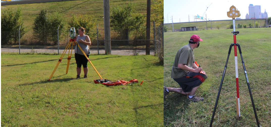
Figures 5 and 6. Drs. Amanda Reignier and Scott Hammerstedt establishing reference points for geophysical survey on TDA property
