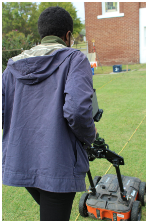
Figure 6. GSSI UtilityScan GPR being operated by TU graduate student Nkem Ike.
